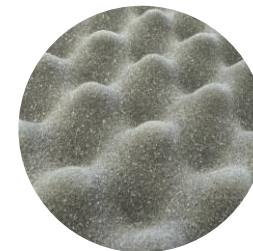
Convoluted acoustic foam interior
